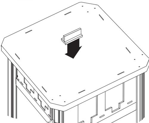
Remove masking from the adhesive strip on the underside of the **Header Clip (K)**. Place **Header Clip (K)** onto the center of the **Top Plate (D)** and insert signage into **Header Clip (K)**.
