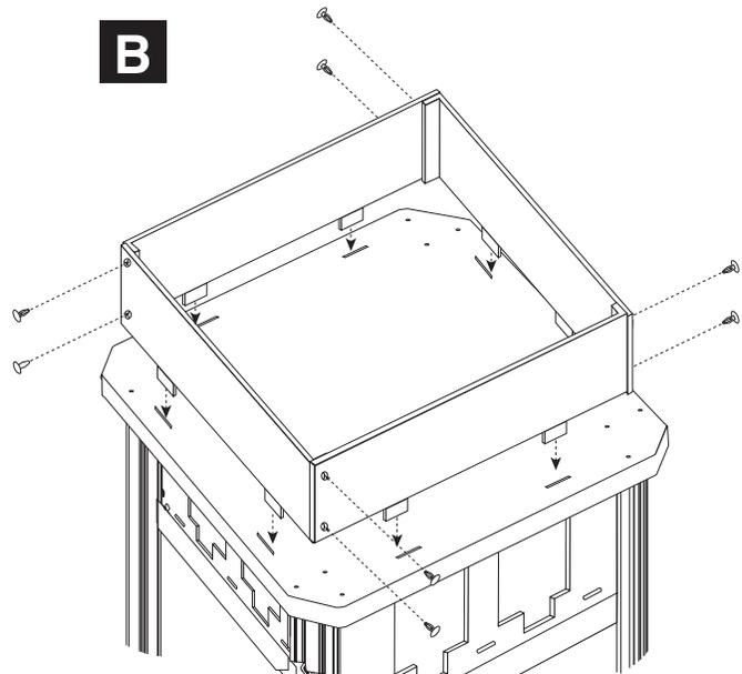
Assemble **Header (G)** with **Push Clips (L)**. Set **Header (G)** into slots on top of **Top Plate (D)**.
