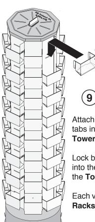
Attach **Racks (H)** by hooking the tabs into the vertical slots in the **Tower Panels (D)**.
