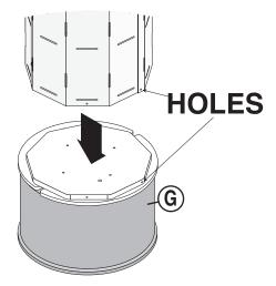
Align corresponding holes and set the Tower Panel Assembly (D) onto the Base (G).
