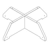
2 Attach Base (J) to X-Base Assembly (K/L) using (4) Connector Bolts (C).
