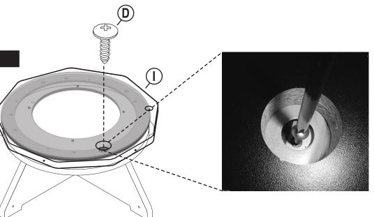
Turn Spinner Plate Assembly (I) 90° to continue attachment to X-Base Assembly, slight positioning adjustment may be necessary to find hole. To attach Spinner Plate (I), use 2nd Short Trusshead Screw (D) through large hole to corresponding hole of X-Base Assembly.
