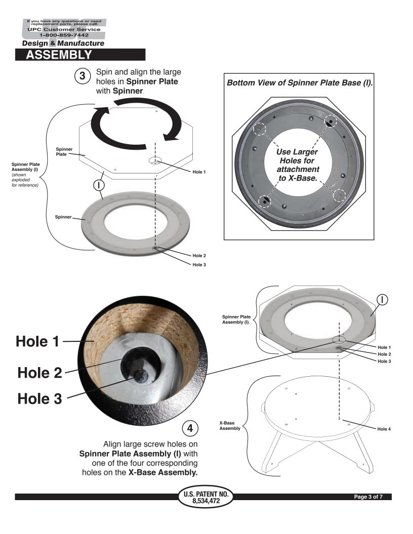
If you have any questions or need replacement parts, please call: UPC Customer Service 1-800-859-7442 **Design & Manufacture** D ASSEM Bl Attach Spinner Plate 5 Assembly (I) to X-Base Assembly by using (1) Short **Trusshead Screw (D)** through large screw hole in Spinner Plate (I) to hole in X-Base Assembly. DO NOT tighten completely!
