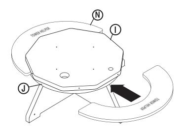
Align corresponding holes and set the Tower Panel Assembly (H) onto the Base Assembly.
