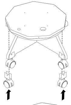
3 Screw Philips Head Screws (A) through Locking Casters (B) into Base Assembly.
