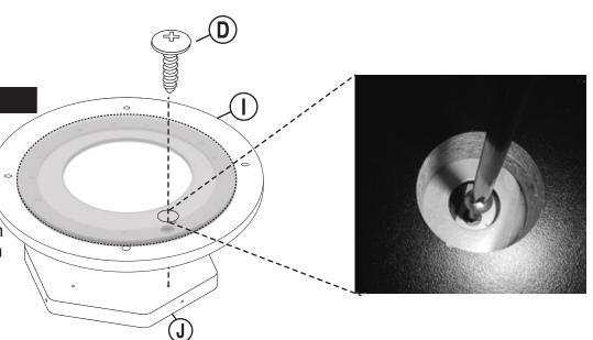
Turn Spinner Plate (I) 90° to continue attachment to Top Plate (J), slight positioning adjustment may be necessary to find hole.
