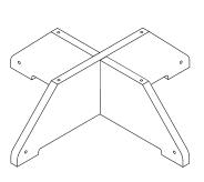
7 Attach Spinner Plate Assembly (I/J) to X-Base Assembly (K/L) using (4) Connector Bolts (C).
