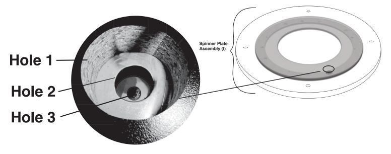
Align largest screw holes on Spinner Plate (I) with one of the four corresponding holes on the Top Plate (J).
