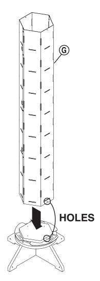
Secure Tower Panel Assembly (H) to Base Assembly at middle holes of Tower Panel Assembly. Attach Tower Panels to Spinner Plate edge with (2) Trusshead Screws (B). DO NOT tighten completely!
