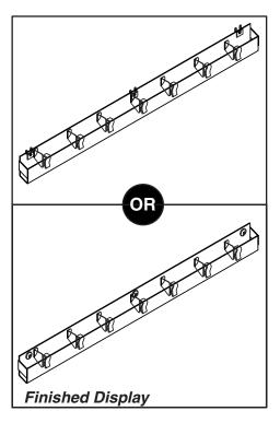
Align hole in **Slatwall Adapter (B)** with back side of hole in **Rack (G)**. Prongs extend back toward Slatwall and up. Attach using **Screw Post (D)** from front and **Nut (E)** on back.
