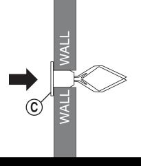
**NOTE:** DO NOT use wall toggler if mounting to a wall stud. Use Wall Toggler for hollow drywall only. Use 3/32" drill bit for any screws drilled directly into studs.
