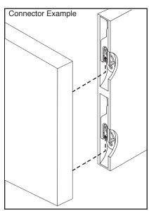
To assemble panels to sides, slide panel down over shoulder screws until they are in line with clip raceway and slide brace down the back of the sides until panel "clicks" into place.
