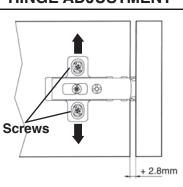
NOTE: If hinges do not align, loosen screws and adjust right to left as needed to align hinge and base plate. Then retighten the screws.
