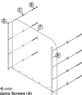
Screw Left Support (G) and Right Support (H) onto Aisle Shield (F) into place using (8) Short Tapping Screws (A) and (8) Finishing Washers (C).
